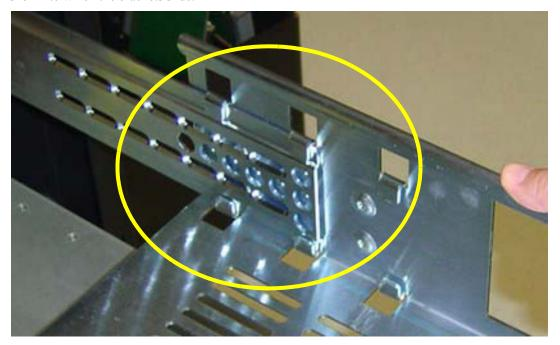
Figure 2-5: Align Shelf with Installed Brackets
